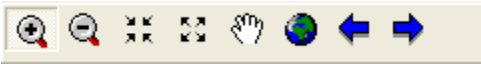
Example of the Map Navigation toolbar holding interactive tools for Zoom, Pan, Full Extent, and Previous Extent.
